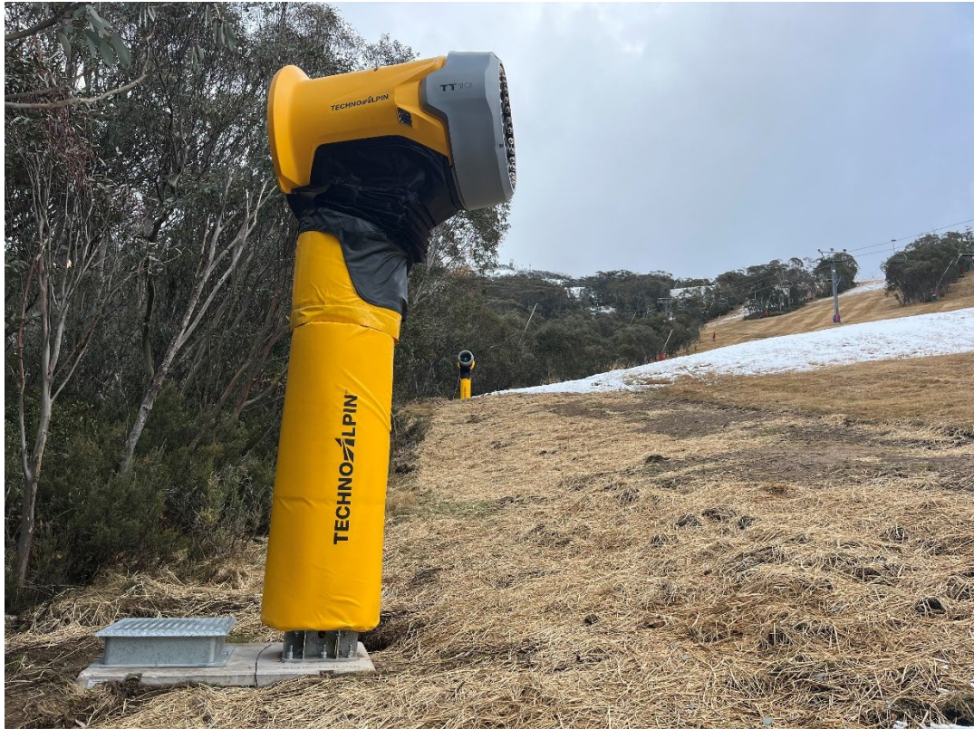
Figure 7: Example of TT10 Fan Gun and Fan Pit
